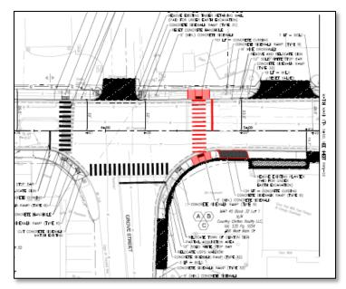
The crosswalk location originally proposed in the 30% design plans would be shifted west to allow for a controlled access driveway onto Route 1 at 56 West Main Street. This change will help maintain the existing traffic flow at the site for deliveries and customer access.
