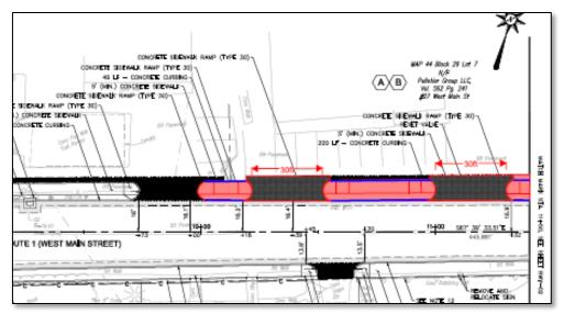
The raised sidewalk in front of 25-27 West Main Street will be moved from the locations proposed in the 30% design plans to maximize the number of parking spaces that can be accessed in the front of the building.
